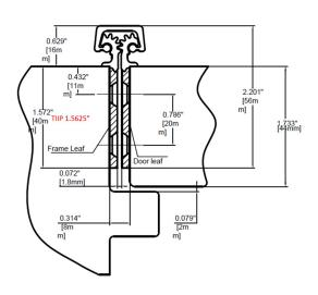
The continuous geared hinges attach to the full height of the door. This distributes the weight of the door along the height of the frame and reduces stress on the hinge which lasts longer than standard butt or mortise hinges, excellent choices for high-traffic entrances at retail, school, hospital, and business sites.
